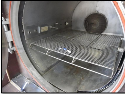
The plug and key (both marked 01) inside the climatic chamber during the dry heat test
